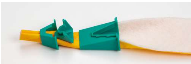
Insert folded fabric and batting strips into part C to fold again. Place part D on the top of the fabric and batting strips and click into with part C.
