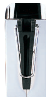
Finished tape width 3/4 in Insert the fabric through the bias tape maker and iron.
